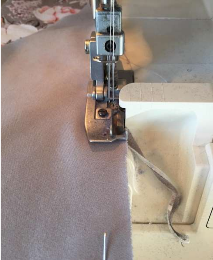
Stitch the shoulders. Knit binding : Stitch one shoulder. Knit bind the neckline. Stitch the other shoulder.
